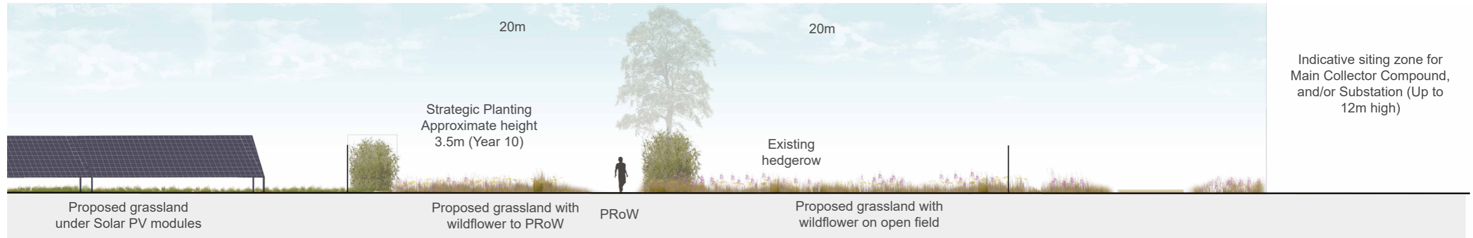
Figure 6.18: Indicative section through PRow Midshires Way
